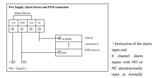
close type). The power out of the alarm sensor can be provided by the DVR(Low current only) or (External alarm power supply)
